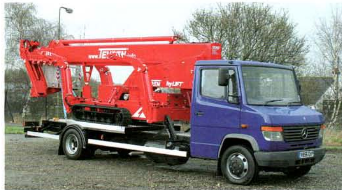
Aspect Access of Harrogate runs this interesting combination of a Teupen Leo30T tracked platform and Mercedes 7.5 tonne Vario truck.
